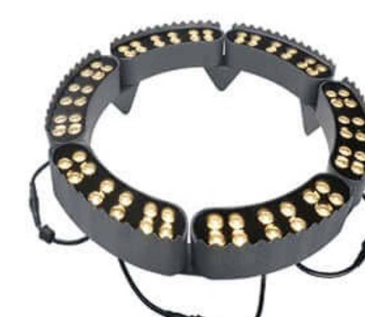
Model: UPW-LTL-020 Product Size: Φ500*H130 MM Power: 72W P.G.: IP65 Led Brand: Bridgelux Input Voltage: 24VDC Material: Aluminium Alloy + Tempered Glass Len's Angle Options: 10°, 15°, 30°, 45°, 60°, 90° Led's Color Options: 2700K, 3000K, 4000K, 5500K, 6500K Red, Green, Blue, DMX Rgb
