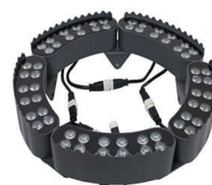
Model: UPW-LTL-018 Product Size: Φ425*H130 MM Power: 60W P.G.: IP65 Led Brand: Bridgelux Input Voltage: 24VDC Material: Aluminium Alloy + Tempered Glass Len's Angle Options: 10°, 15°, 30°, 45°, 60°, 90° Led's Color Options: 2700K, 3000K, 4000K, 5500K, 6500K Red, Green, Blue, DMX Rgb
