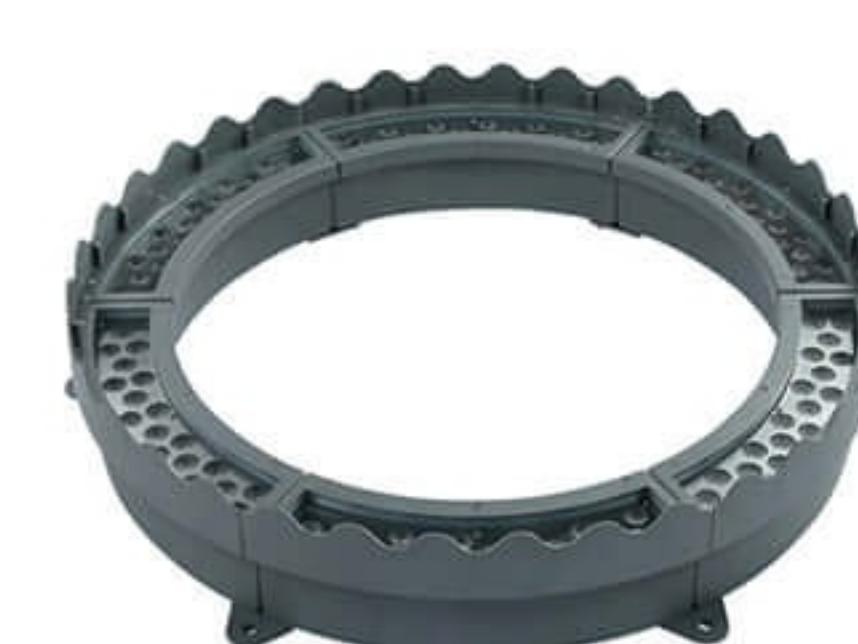
Model: UPW-LTL-034 Product Size: Φ665*H160 MM Power: 108W P.G.: IP65 Led Brand: Bridgelux Input Voltage: 24VDC Material: Aluminium Alloy + Tempered Glass Len's Angle Options: 10°, 15°, 30°, 45°, 60°, 90° Led's Color Options: 2700K, 3000K, 4000K, 5500K, 6500K Red, Green, Blue, DMX Rgb
