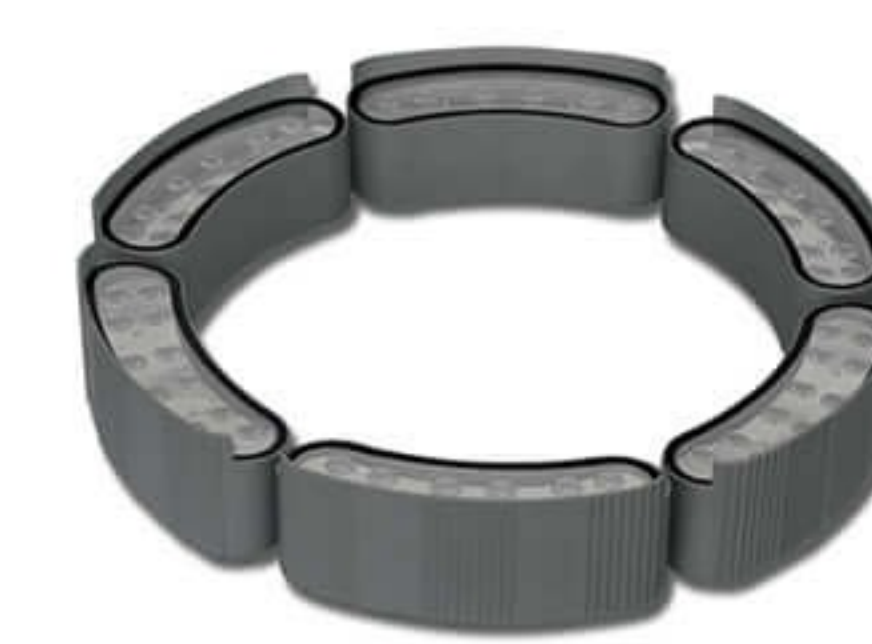
Model: UPW-LTL-019 Product Size: Φ470*H130 MM Power: 72W P.G.: IP65 Led Brand: Bridgelux Input Voltage: 24VDC Material: Aluminium Alloy + Tempered Glass Len's Angle Options: 10°, 15°, 30°, 45°, 60°, 90° Led's Color Options: 2700K, 3000K, 4000K, 5500K, 6500K Red, Green, Blue, DMX Rgb
