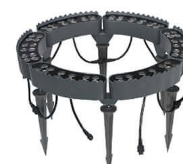
Model: UPW-LTL-021 Product Size: Φ500*H270 MM Power: 72W P.G.: IP65 Led Brand: Bridgelux Input Voltage: 24VDC Material: Aluminium Alloy + Tempered Glass Len's Angle Options: 10°, 15°, 30°, 45°, 60°, 90° Led's Color Options: 2700K, 3000K, 4000K, 5500K, 6500K Red, Green, Blue, DMX Rgb
